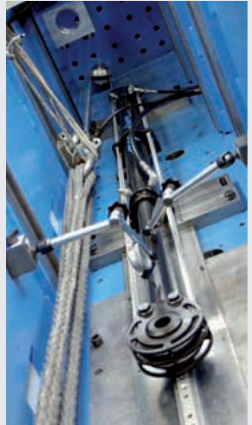
Bench test, with a length of 4200 mm, has been thought to test at 100% every size of Cariboni's ram.
