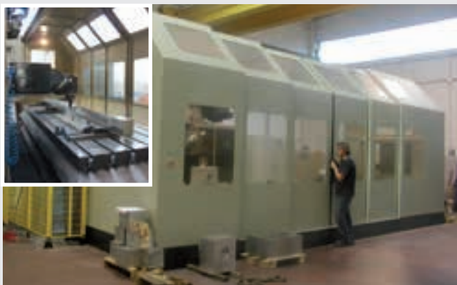
The "Tiger - TLM 4" CNC milling machine is the biggest machine of the firm. The birotating head works over a volume of 4000x1200x1500 mm and has a target power of more than 28 kW. Fins and bulbs are machined out here as the biggest parts for the custom arrangements.
