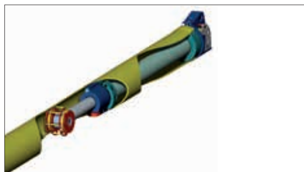
The mainsheet is controlled by a smaller unit installed inside the boom.
