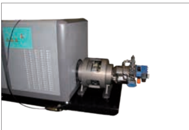
Rexroth pump assembled with custom clutch on 27kW Mastervolt generator PTO. Flow rate = 67.5 lit/min Max pressure = 250 bar
