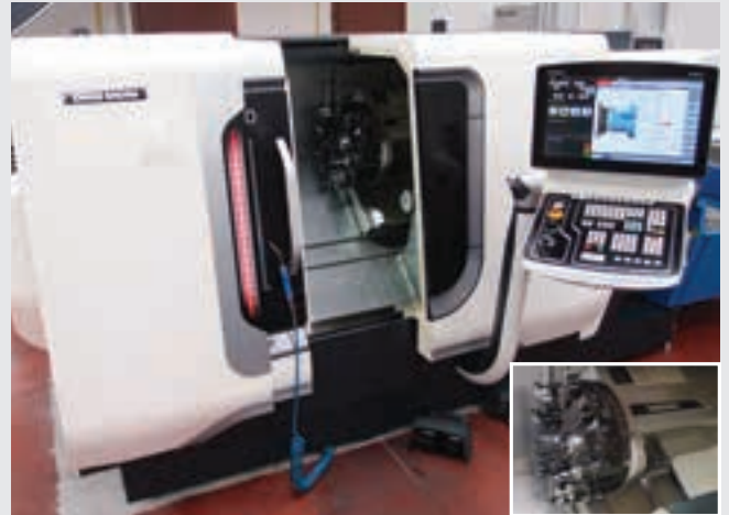
DMG Mori - CTX Alpha 500 - CNC lathe and milling machine, 4 axis. It is equipped with motorised tools, integrated mandrel motor and Y axis. It enables also off-centre turning and milling.
