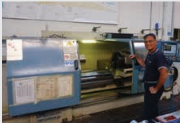
The "Zanoletti" medium size 5 axes CNC lathe. Small and medium size cylinder parts are machined out here.
