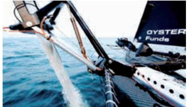
Double acting cylinder with integrated linear sensor to control foil angle of 32' race catamaran.
