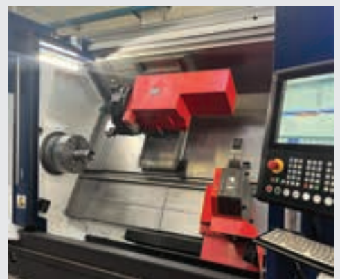
Emco Maxx Turn 110 – CNC lathe and milling machine, 4 axis. It is equipped with motorised tools, integrated mandrel motor and Y axis. Max Ø: 560mm. Max length: 3520mm.
