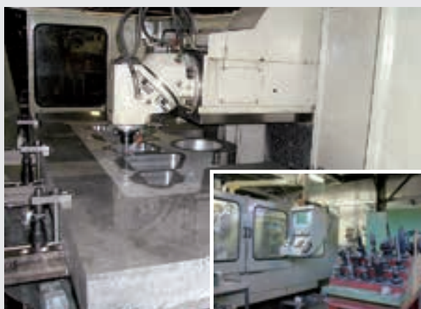
The "Tiger" CNC milling machine is one of the most reliable machine of the firm. The "Momac" lathe machine is used to produce small-medium pieces up to 400 x 1000 mm. Pins, small cylinder pistons and parts of manual components are machined out here
