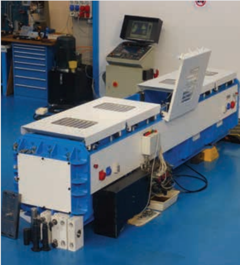
Bench test, with a length of 4200 mm, has been thought to test at 100% every size of Cariboni's ram.
