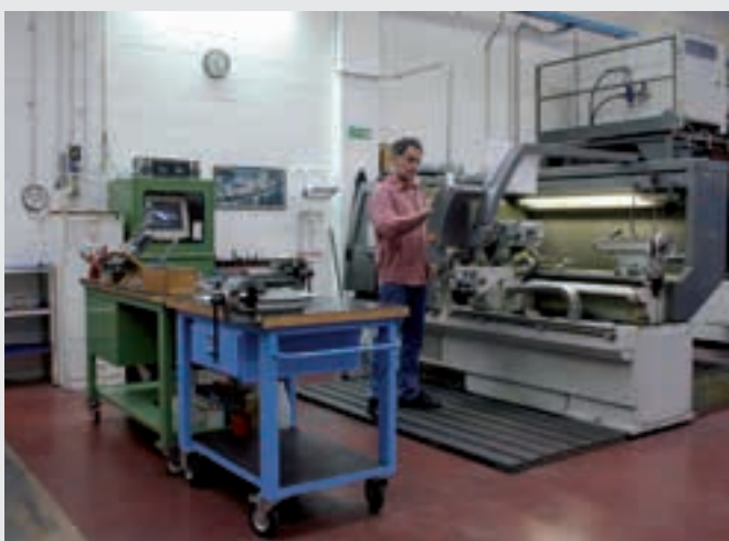
The "Momac" lathe machine is used to produce small-medium pieces up to 400 x 1000 mm. Pins, small cylinder pistons and parts of manual components are machined out here.
