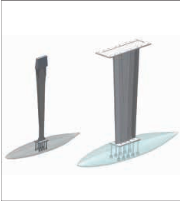
The fin on the left is CNC milling machined from a forged block to obtain the right shape. The one on the right is a welded fin made of Weldox.
