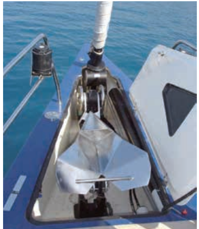
Anchor stowing motor
