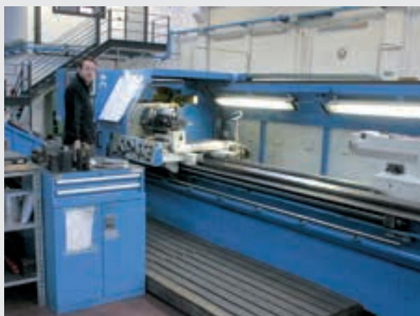
The "PBR" is the biggest lathe machine of the firm. It can machine tubes up to 3500 mm length with a diameter of 700mm. Big Magic Trim tube, rods and big cylinders components are made by this machine.
