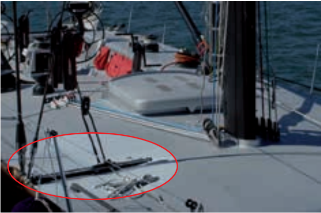
This double acting cylinder, closed to traveler arrangements is installed on a 90' race-cruiser yacht. It controls the jib car by two sheets and it is squeezed under the car track in a very small room.
