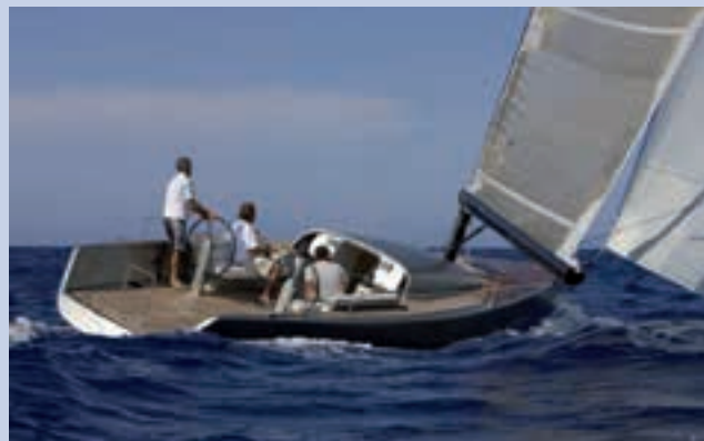
B42 day sailing yacht. Halyard, main track and mainsheet are all driven by Cariboni's aluminium rams.
