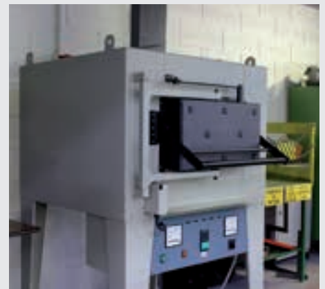
The oven for the heat treatment of special parts (like bolts for the canting keel systems). It can warm up pieces up to 1100°C.
