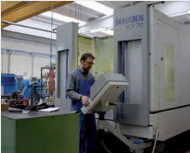
The "Mikron" small CNC milling machine is mainly used for the production of manual system components as pump, valves and other small parts. It is a 5 axes mill with a working space of 710x500x500 mm.
