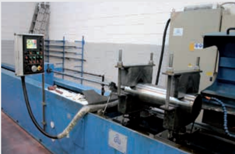
The "Lappatrice" is our CNC lapping machine used for every type of cylinder or Magic Trim tubes. It can handle up to 4.5 meter of tube with an internal diameter of 400mm!
