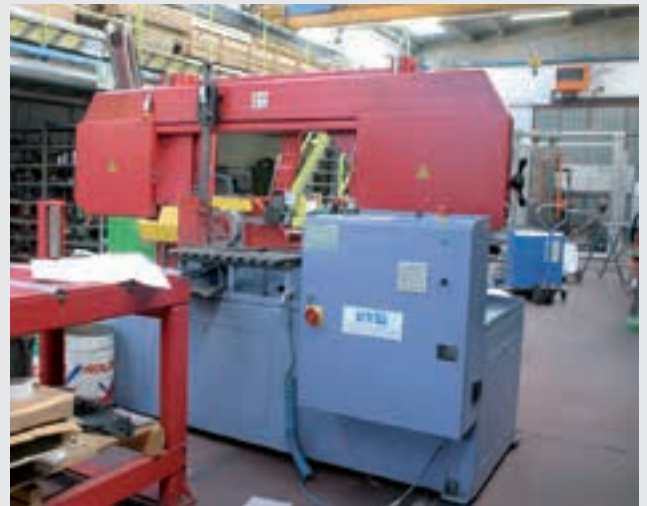
The chain sawing cuts every size of pieces (aluminum, steel and titanium).
