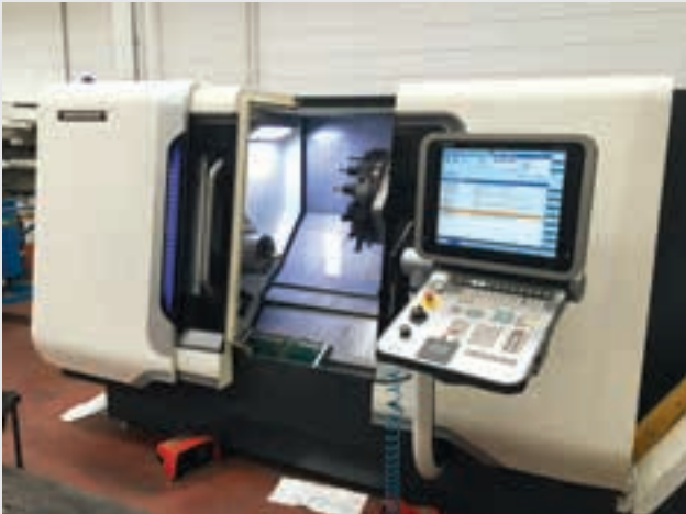
DMG Mori - CTX Beta 800 - CNC lathe and milling machine, 4 axis. It is equipped with motorised tools, integrated mandrel motor and Y axis.
