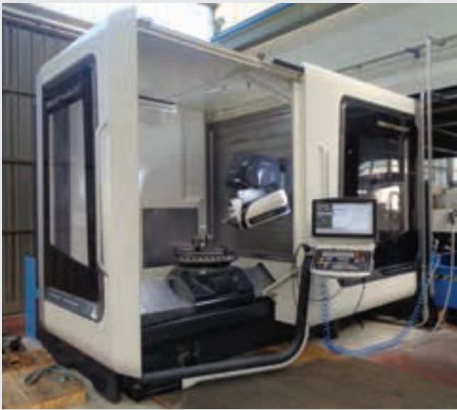
DMU 90 P duoBLOCK – Five axis simultaneous machining with 900mm X-axis, 1050mm Y-axis, 850 z-axis. 15.000rpm speedMASTER spindle and a tool magazine with 60 positions.
