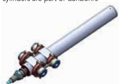
Titanium twin cylinder: n.2 double acting cylinder move together in a common tube. Bore (each): 25mm Stroke: 190mm Working pressure: 700 bar Extreme light weight and compact design.
