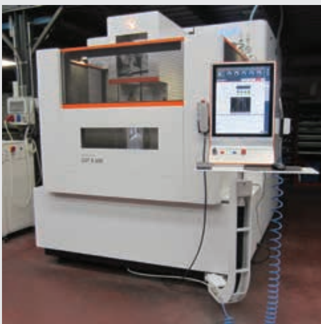
GF Machining Solutions CUT E 600 – With 600 X-axis, 400 Y-axis, 350 Z-axis, wire 0,25mm max taper angle 30°/56mm
