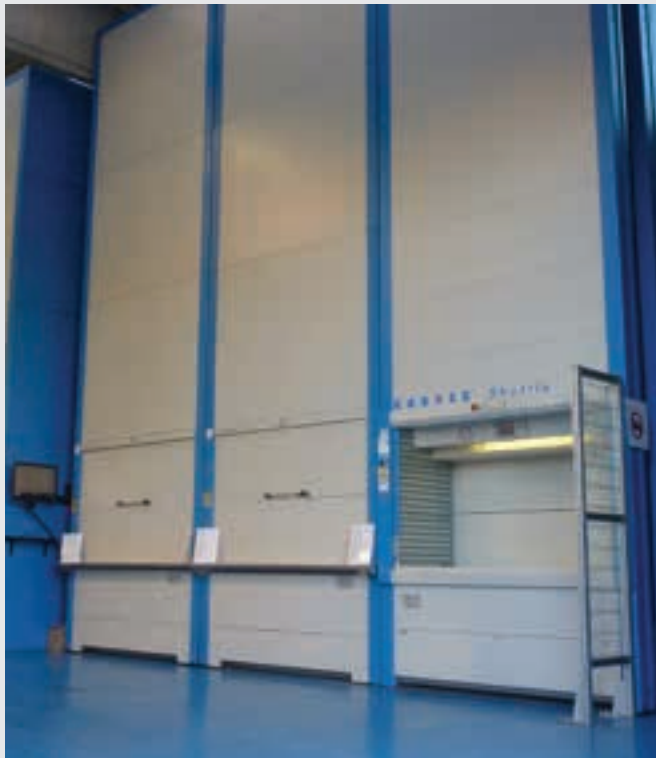
Kardex. Automatic warehouses. Seals, parts and tested products are all stored here managed by a software.
