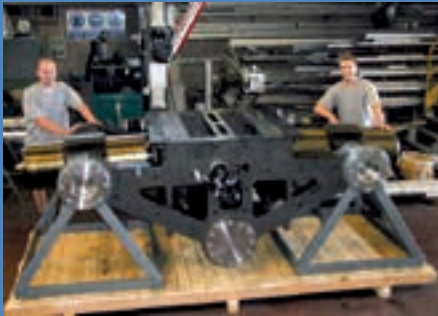
Cariboni's keel system with frame for a 105' sloop. This kind of system is fully tested in the firm before shipping.
