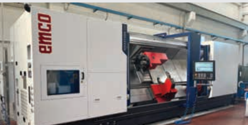
Emco Maxx Turn 110 – CNC lathe and milling machine, 4 axis. It is equipped with motorised tools, integrated mandrel motor and Y axis. Max Ø: 560mm. Max length: 3520mm.
