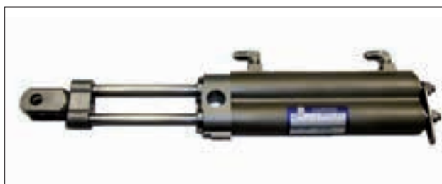
Titanium twin cylinder: n.2 double acting cylinder move together in a common tube. Bore (each): 25mm Stroke: 190mm Working pressure: 700 bar Extreme light weight and compact design.
