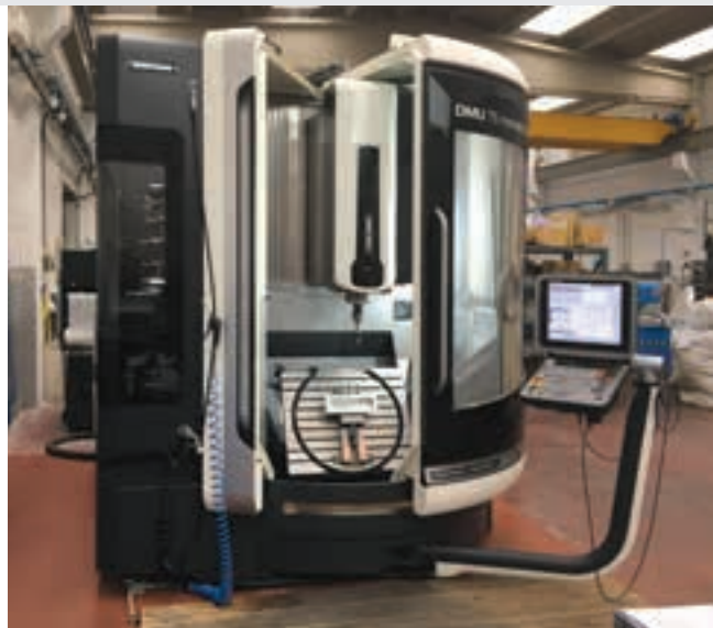
DMU 75 - Five-axis simultaneous machining with 750mm X-axis traverse (75:750mm), 20.000 rpm speedMASTER spindle and a tool magazine with 60 positions.
