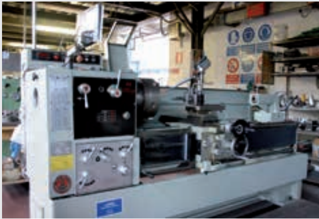
The 2 lathe machines are used to produce special tools for our products and for easy adjustments on the test components.
