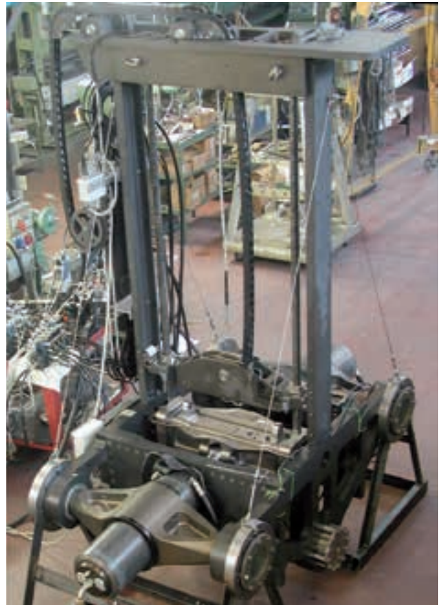
MAIN FEATURES for a 115' racer: Max canting angle: 35° Bulb weight: 11000 kg Fin weight: 400 kg Distance Bulb CG – Axis: 5200 mm Distance Fin CG – Axis: 2000 mm Lifting stroke : 1770 mm Dimensions: 1150x2700x3020 mm Weight: 1500 kg
