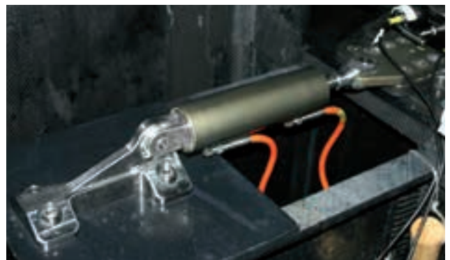
Double acting cylinder to control the mast base position. Made of aluminium, rod and tube terminal made of 17-4PH.
