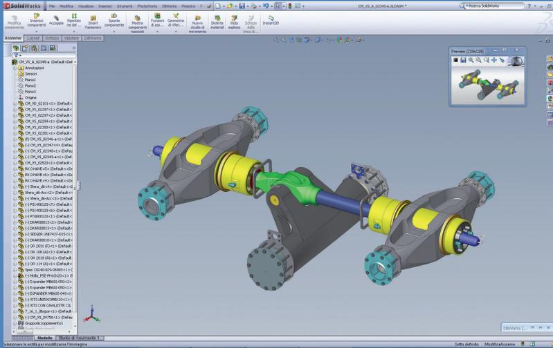
The canting keel feature dramatically improves the righting moment of the boat allowing more power for race yachts or more comfortable sailing for cruisers.
